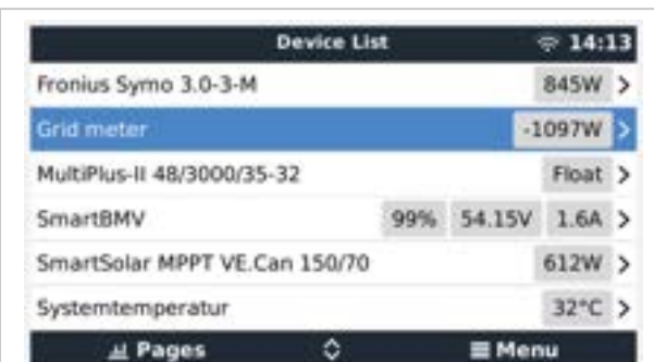
Or configured to measure energy consumption from the grid
