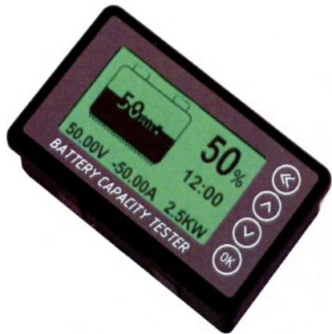
BM Series Current Battery Capacity Display Coulomb counter
