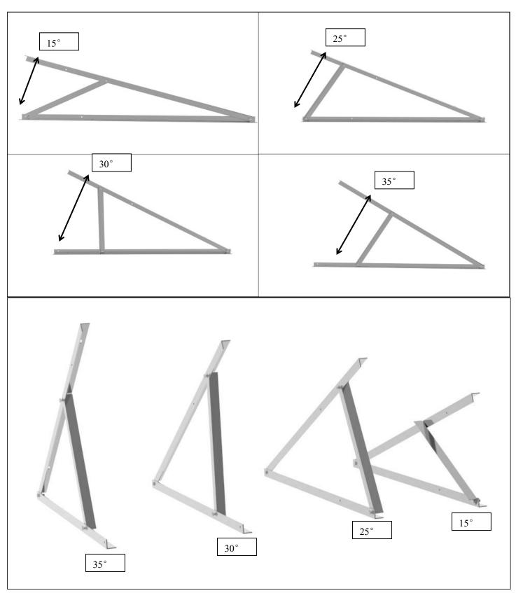
2. Install two angles to the tri-bracket with the bolts and nuts.
